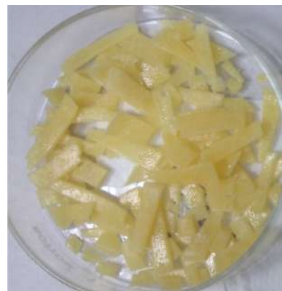
Figure 7: Sliced pieces of solvent cast rosin composite film in a Petri dish ready for bio-extrusion.
