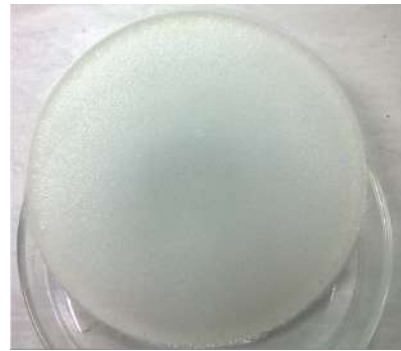
Figure 6: A solvent cast rosin composite film in a Petri dish.
