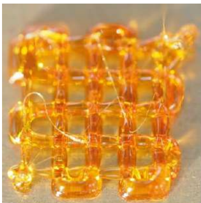
Figure 5: A two-layered rosin scaffold printed at 135 °C.
