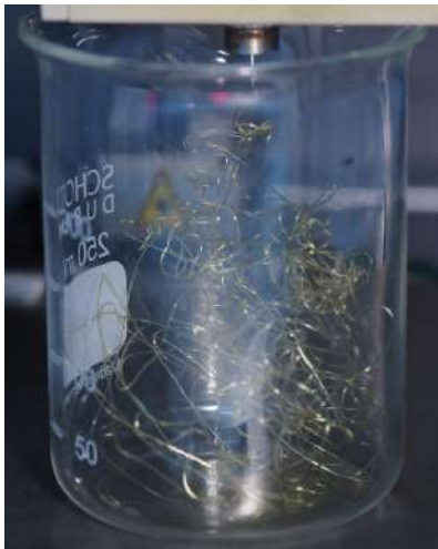
Figure 4: Extruded rosin filaments at 80 °C.
