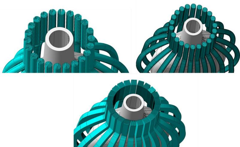
The CFD (computer fluid dynamics) simulations shows it is possible to increase cooling efficiency off the mould. Since the cooling channels are not axial it is possible to identify mould volumes that don't interfere in cooling of the mould, so these material volumes can be replaced by lattice geometries, reducing weight, production times and maintaining structural integrity.
