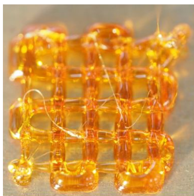
Figure 5: A two-layered rosin scaffold printed at 135 °C.
