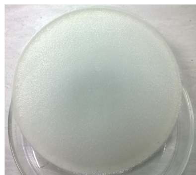
Figure 6: A solvent cast rosin composite film in a Petri dish.
